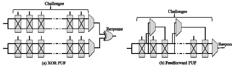
**Fig. 11.** (a) An arbiter PUF with added XORing of two arbiter outputs; (b) Feedforward PUF.
