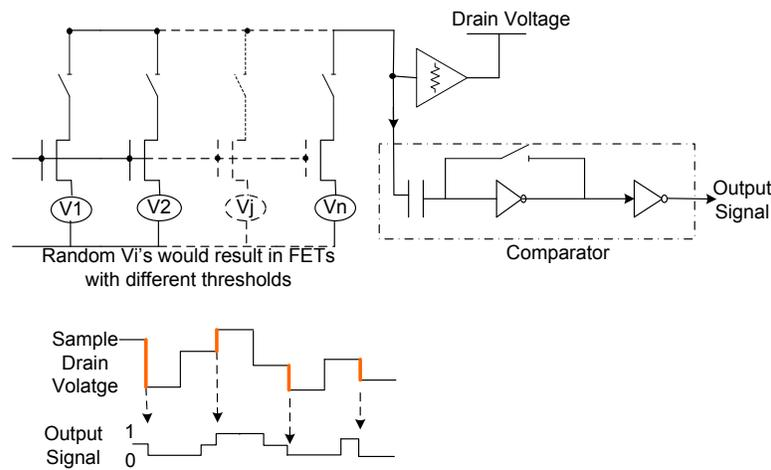
**Fig. 6.** Array of ICID transistors producing a sequential random voltage proposed in [58].
