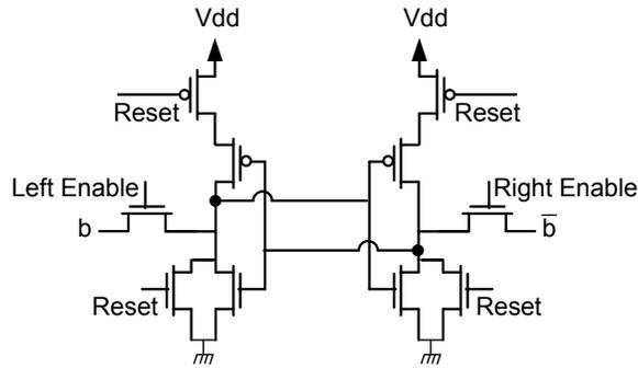
**Fig. 7.** The positive feedback loop created by the cross-coupled NOR (NAND) gates is used for storing a 0 or a 1 in SRAM-like memory structures.
