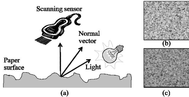
**Fig. 4.** (a) Scanner produces different images of the paper surface based on the page orientation. The light seen at the sensor depends on the angle between the surface normal and the light source; (b) A region of the document can be scanned from top-to-bottom; and (c) The same document region can be scanned from left-to-right. The 3D texture can be estimated by combining (b) and (c) (Figure inspired by studies in [28]).
