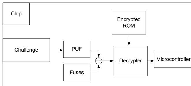
**Fig. 8.** A POK built by using a Strong PUF proposed in [2].
