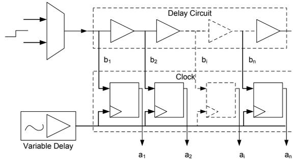
**Fig. 12.** The glitch PUF architecture samples the glitches on the path and the arrival of a glitch compared to a clock signal generates the response bits in the FFs [79].
