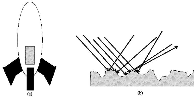
**Fig. 3.** (a) A thin, random layer of light scattering particles sprayed on the missiles. (b) Illuminating the surface from different angles would generate different inference patterns.
