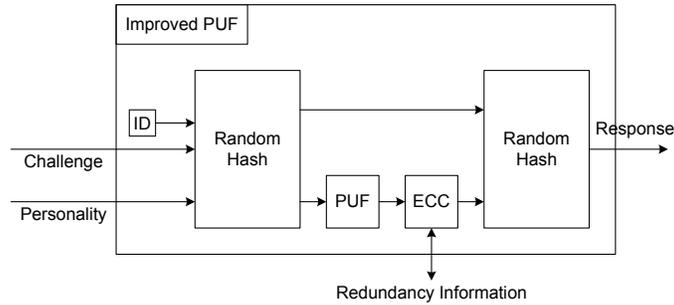
**Fig. 13.** An example architecture for a controlled PUF proposed in [70].
