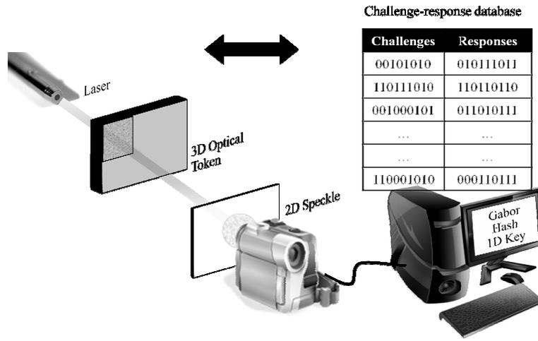
**Fig. 9.** A 3D inhomogeneous transparent plastic token being optically challenged (illuminated under different angles and points of incidents) and produces an output in form of an interference pattern. The output is hashed to produce a 2D image, which is in turn filtered by a multiscale Gabor transform to produce a 1D key as proposed in [69].
