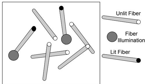
**Fig. 5.** Examples of randomly placed, fixed-length fibers. The square demonstrates the embedding substrate. Three fibers lit by spot illumination light as described in [33].
